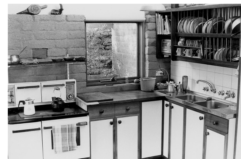
Kitchen with slow combustion wood stove, blackwood bench, cupboard doors and plate draining rack over sink. Warming rack over stove used for sprouts, yoghurt and drying. Note: third tap over sink is gravity fed from rainwater tank.
