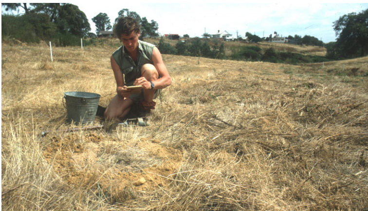
David testing soil from auger holes in main dam site for clay content, February 1986. Higher stake marks where dam wall will meet the Olver Street reserve while the lower stake marks the top water level. The gentle form of the drainage line (visible following tractor slashing of the site) results from filling of the eroded water course with earth moved by previous land owners.
