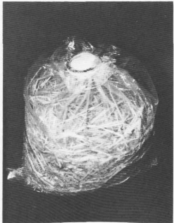
Figure 110 Autoclavable plastic bag and microporous filter disc, known in the Orient as the Space Bag.
