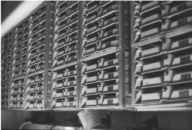
Figure 5. Heath Vertical egg-incubation system.
