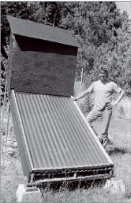
Jack's solar convection fruit dryer. Trays inside black box hold fruit.
