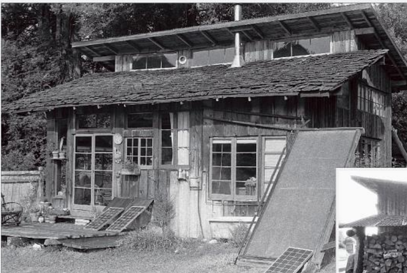
The house Kate now lives in, showing solar collector for outdoor shower and photovoltaic solar panels that charge batteries
